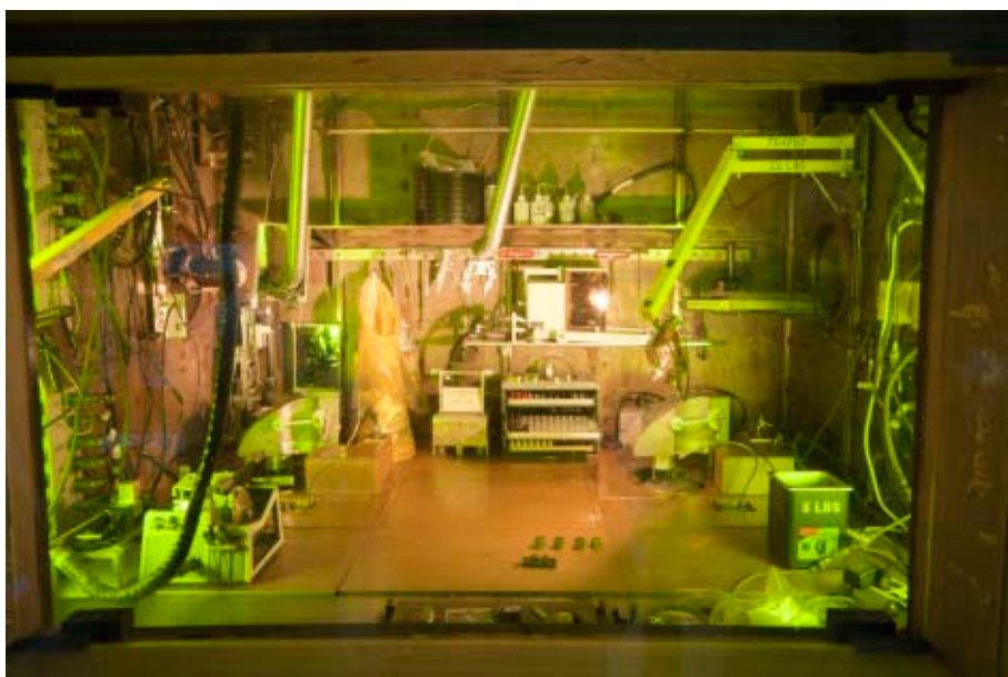
Figure 1 HFEF containment box where capsules are disassembled, catalogued and frequently stored prior to retrieval.
