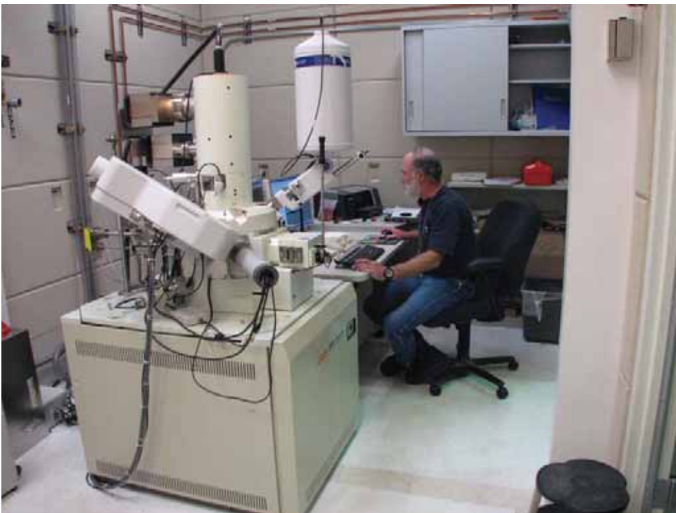
JEOL Field Emission Scanning Electron Microscope with EDS, WDS, and EBSD
