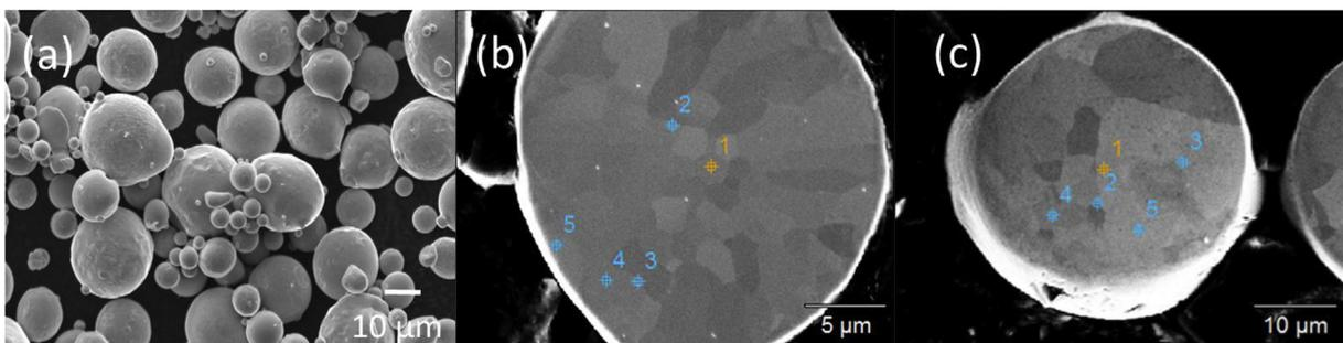
Fig. 3. SEM micrographs of the gas atomized 14YWT ODS powder in (a) as-received powders showing a range of powder particle sizes (b) cross-section image of powder from the <20  $\mu\text{m}$  size range, (c) cross-section image of powder from the 20  $\mu\text{m}$ –44  $\mu\text{m}$  size range. The cross-sectional images also indicate the points where EDS analysis was performed for data for shown in Fig. 4.
