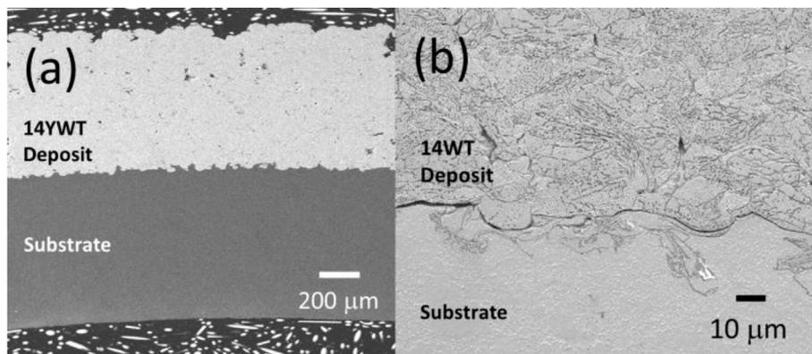
**Fig. 7.** Cross-sectional SEM image of tubular deposition of 14YWT (a) showing deposition on tubular mandrel substrate (b) high magnification image of deposit and substrate interface after etching with Kalling's reagent.
