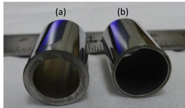
**Fig. 8.** Photograph of 14YWT ODS tube after surface polishing showing (a) ODS deposit with the 6061-T6 Al-alloy substrate tube, and (b) after dissolution of the inner Al-alloy substrate tube showing free standing ODS tube.
