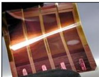
PAS can address important questions in a variety of polymers, such as PEMs and OPVs for energy applications, where free volumes play critical roles. For example, organic semiconductors are promising candidates for low-cost, flexible electronics that can be deposited by a simple printing process. The nanostructure of the OPV materials is believed to have profound impact on the final device performance. However, their exact correlation is still topics of debate. Since PALS is
