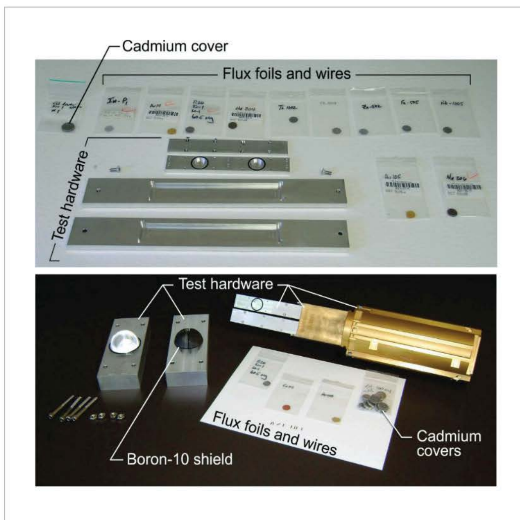
Figure 29. Representative flux wires, flux foils and test hardware used at INL [33].
