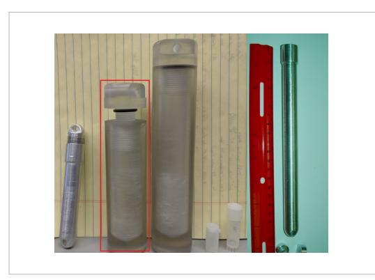
Figure 5. Available capsules for NRAD drop-in irradiation. (Left) Aluminum capsule with screw cap, also available with weld caps (right). (Middle) Nylon or polyethylene capsules of various dimensions, polyethylene vials of 0.6-in. diameter by 2-in. long and other available dimensions for containing fuel and materials, and double-capsulated in capsules shown on the left and middle.
