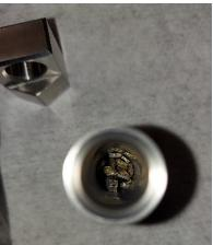
Figure 6. An example of Swagelok capsule that was used for TRISO particles, TRISO compacts, structural materials.
