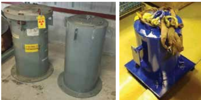
(Top) Westinghouse shipping containers warehoused for radiological material transport / (Bottom) Westinghouse shipping casks for transporting highly activated material specimens
