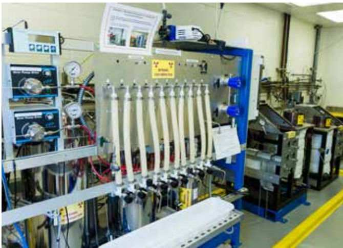
Custom-built test rig for evaluating impacts of zinc addition to light water reactor coolant on stress corrosion crack resistance
