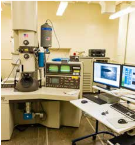
FEI CM30 300-KV TEM equipped with an Oxford Instruments Si Li EDS system
