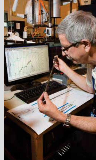
Visual examination of fuel rod simulant after exposure in the WALT Loop
