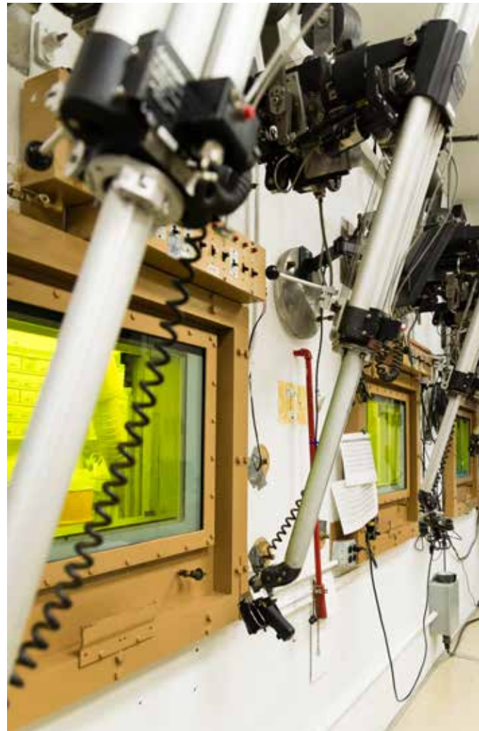
SEM hot cell viewing window with manipulator
