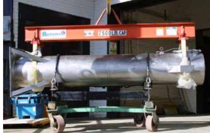
Surveillance capsule cask with integrated stand for shipping and receiving long capsules
