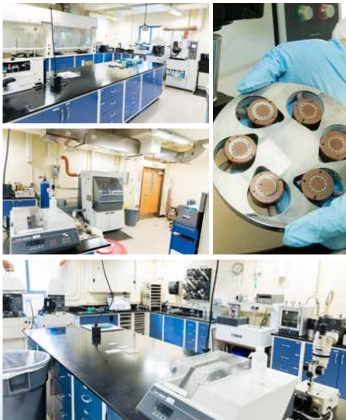
Metallographic preparation laboratory with example of as-polished samples
