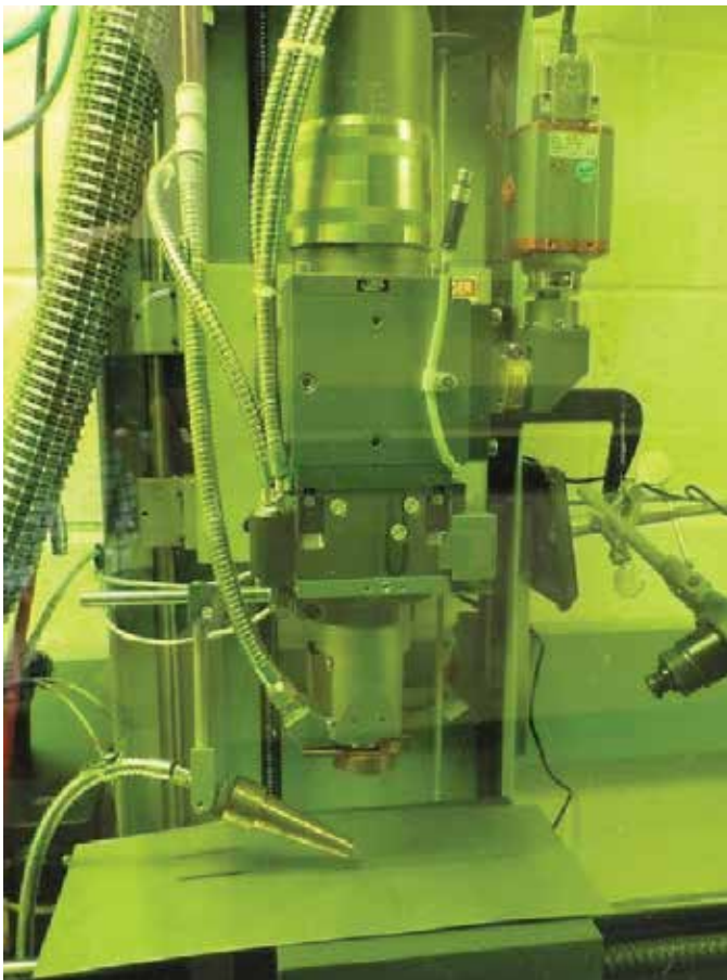
Neodymium-doped yttrium aluminum garnet (Nd:YAG) laser welding head with video feedback system, air knife and multi-axis positioning
