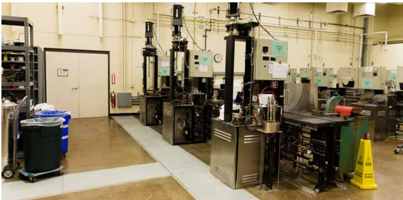
Autoclaves equipped with load frames
