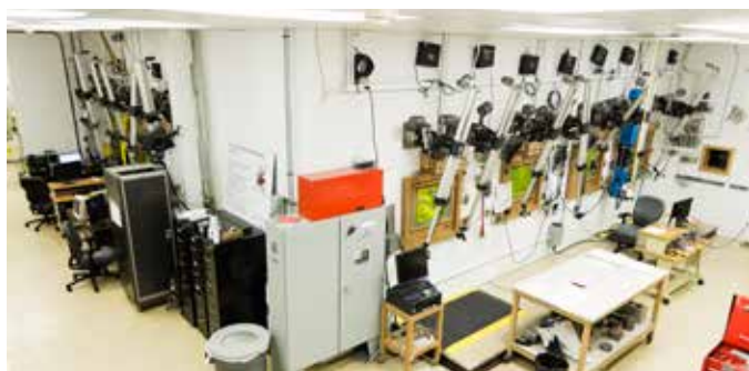
High-level hot cell with four remote handling stations (right) and low-level hot cell with three remote handling stations (left)
