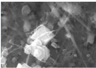
Oxide deposits on the inside diameter surface of an Alloy 600 steam generator tube
