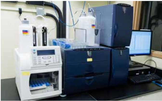
Thermo-Dionex ICS-5000 Anion/Cation system with autosampler
