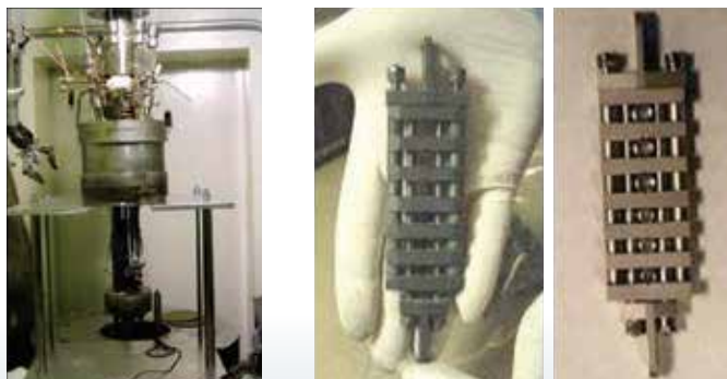
(Left) Westinghouse's In-Cell Crack Growth Rate Test Assembly. (Right) Test fixture for loading six O-ring specimens for Internal Association for Six Sigma Certification (IASCC) initiation testing.
