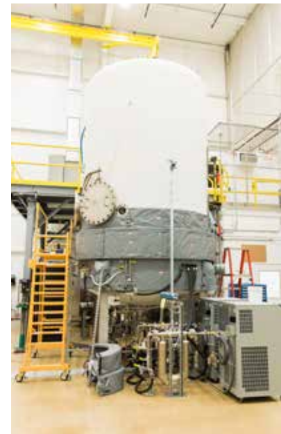
Condensate return testing tank and measurement equipment
