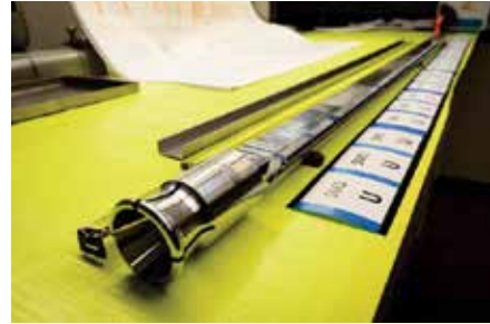
Fabrication and assembly of surveillance capsules for Westinghouse's newly constructed plants in China
