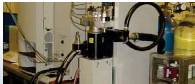
Modified LECO RHEN-602 H-Analyzer (prior to hot cell installation)
