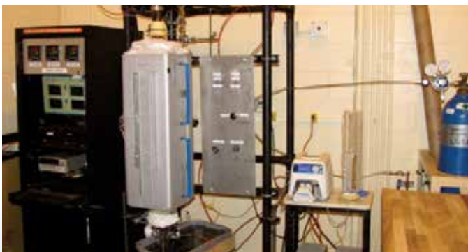
High-temperature steam oxidation equipment used for evaluating LOCA effects on fuel cladding materials
