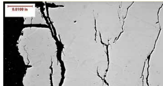
Transgranular stress corrosion cracking in austenitic stainless steel
