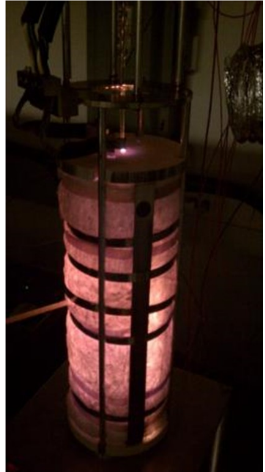
Bench Test of High-Temperature Furnace
