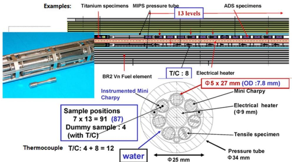
Figure 10: picture and schematic of the MISTRAL capsule.
