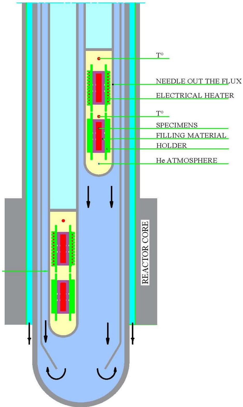
Figure 8: schematic of the LIBERTY device.
