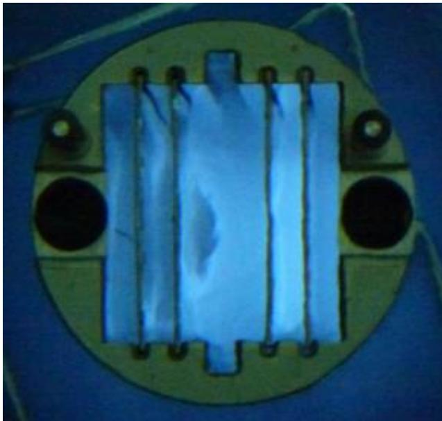
**Figure 5: Picture of the FUTURE type basket for irradiation of 4 MTR fuel plates. The central aluminum plate, containing activation dosimeters, is removed in these pictures.**
