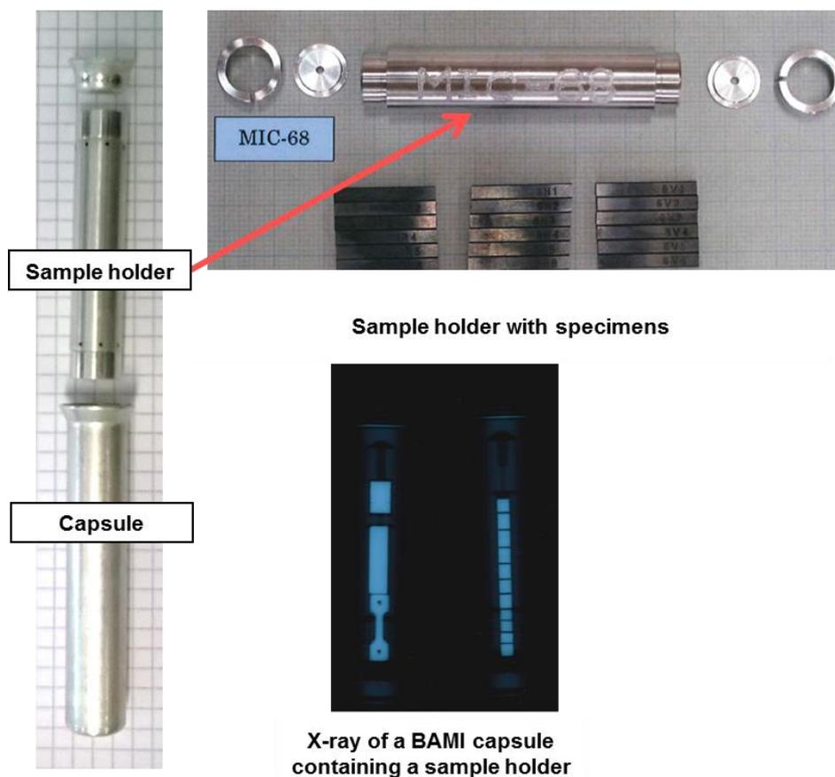
**Figure 6: BAMl capsule with typical sample holder and samples.**
