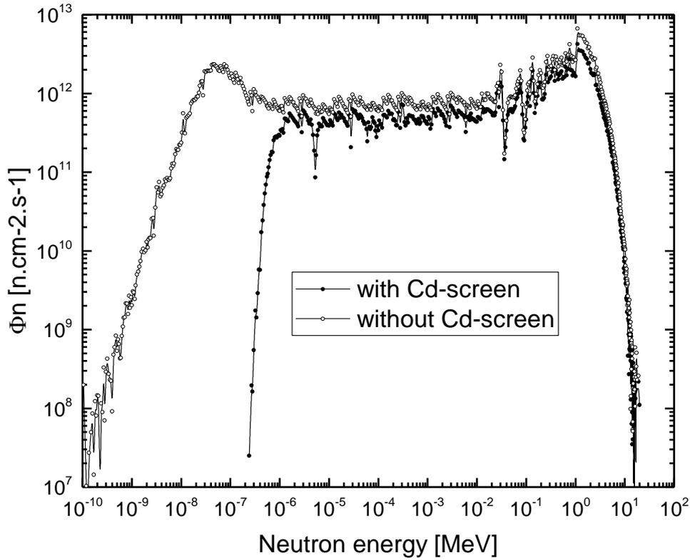
Figure 2: neutron spectrum typical for the BR2 reactor.
