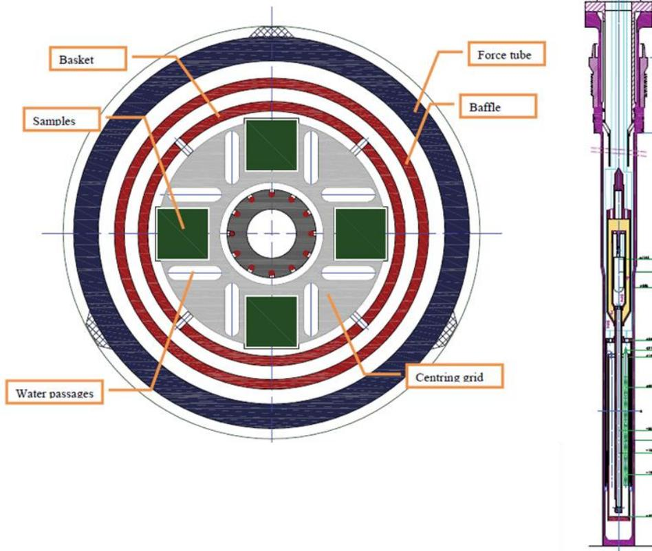
Figure 9: schematic of the RECALL device.
