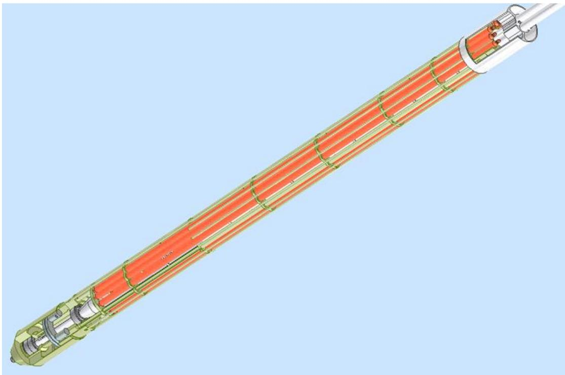
**Figure 7: drawing of the ROBIN device, showing 3 of the 9 sample holders.**
