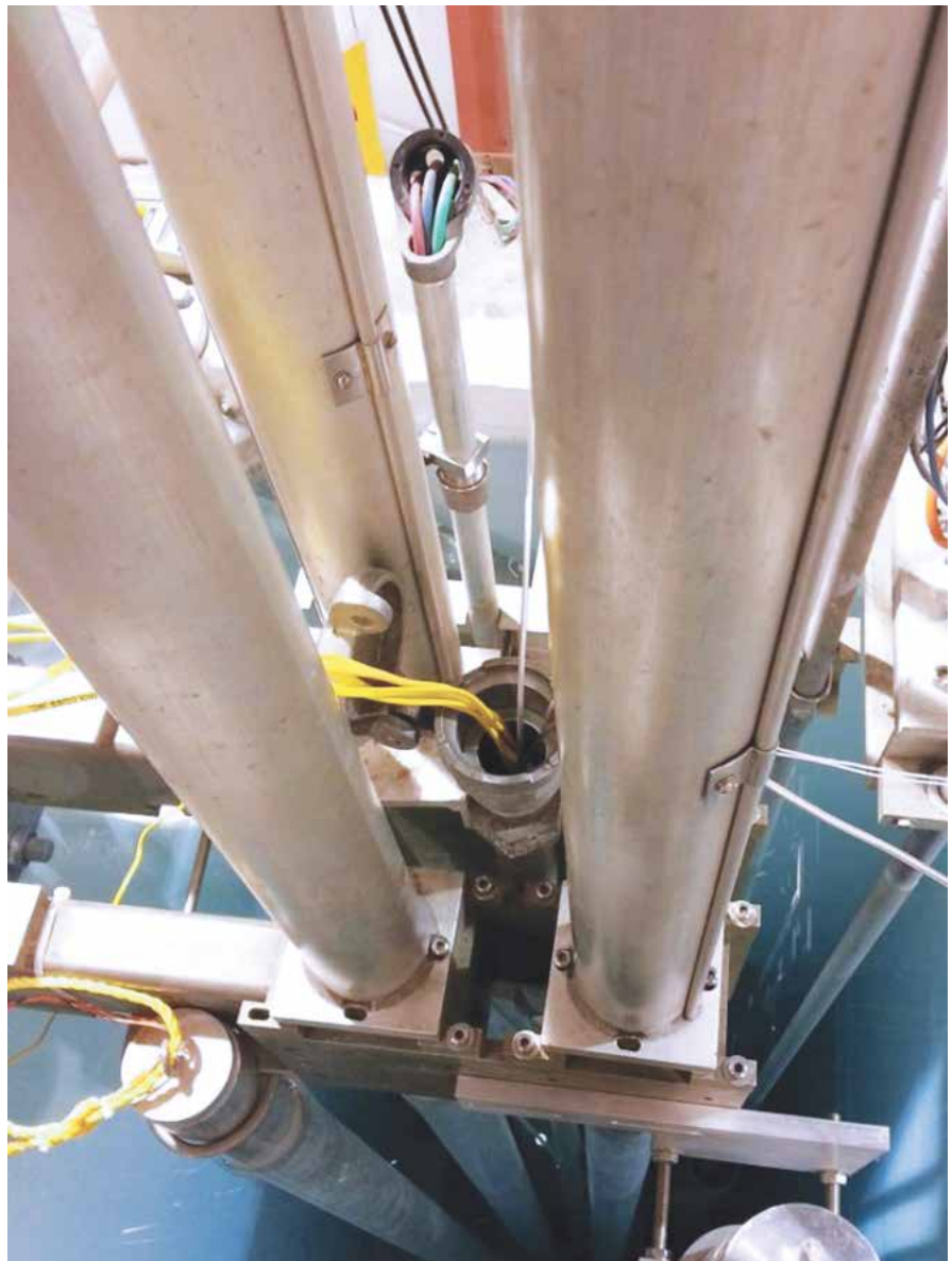
Figure 1. Experiment installed in the central irradiation facility of The Ohio State University Research Reactor.
