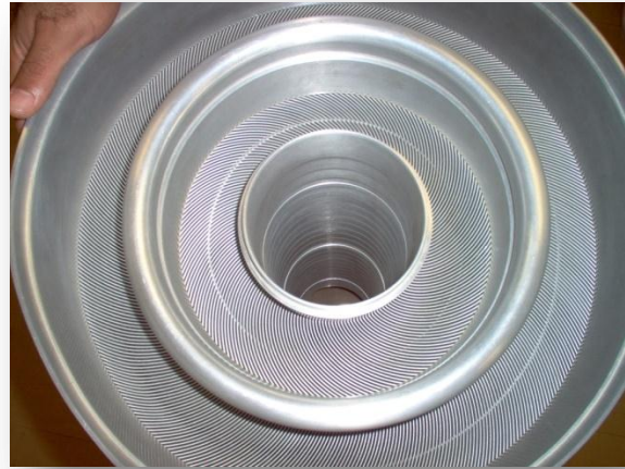
Figure 7: Top View of a HFIR Fuel Bundle
