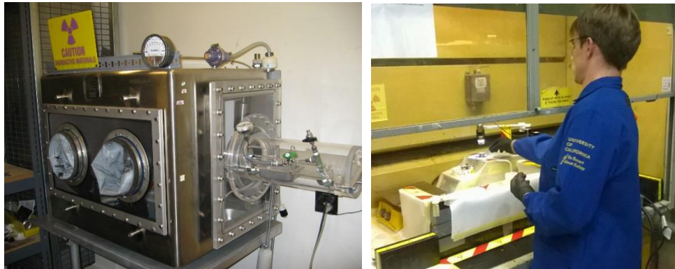
Figure 1: Stainless steel glove box for radioactive sample preparation. The box contains an Allied slow speed cut off saw, a Buhler minimet polisher, and a hot plate. The glove box is located in a separate lockable part of the nuclear materials laboratory to ensure access only to trained users a). Further sample preparation on activated materials can be performed in the certified hoods as shown in b).
