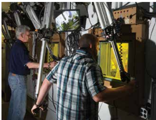
Operators use manipulators to perform work at the Westinghouse Hot Cell Lab.
