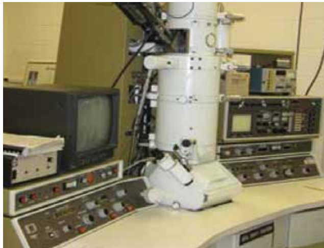
A JEOL 200CX TEM equipped with EDS and scanning system, and an electro-polisher and dimpler at the Characterization Laboratory for Irradiated Materials, located on the UW campus in Madison, Wisconsin.
