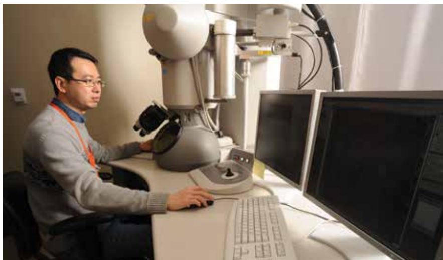
Transmission electron microscope, one of many PIE capabilities in the Microscopy & Characterization Suite (MaCS) at the Center for Advanced Energy Studies in Idaho Falls, Idaho.
