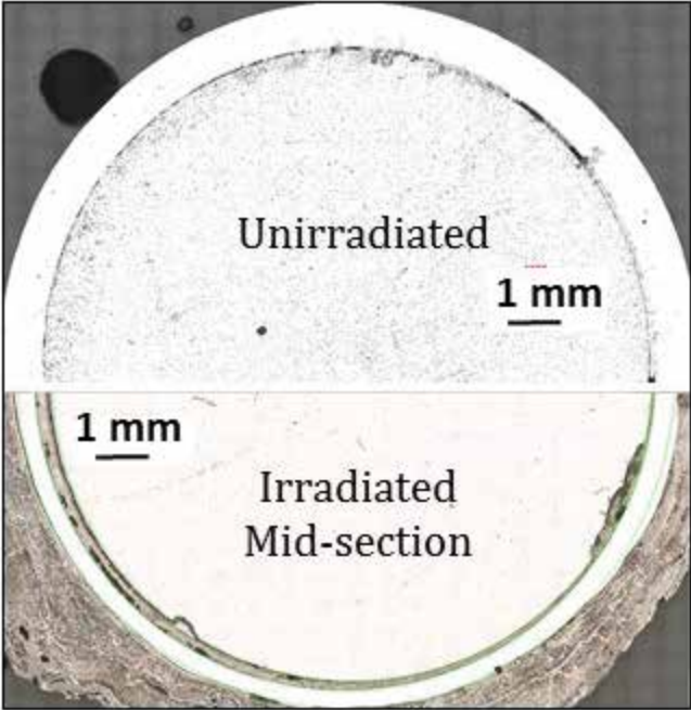
Figure 1. Mid- and lower-level cross-sectional optical images of irradiated fuel rodlet as overlapped to unirradiated fuel.
