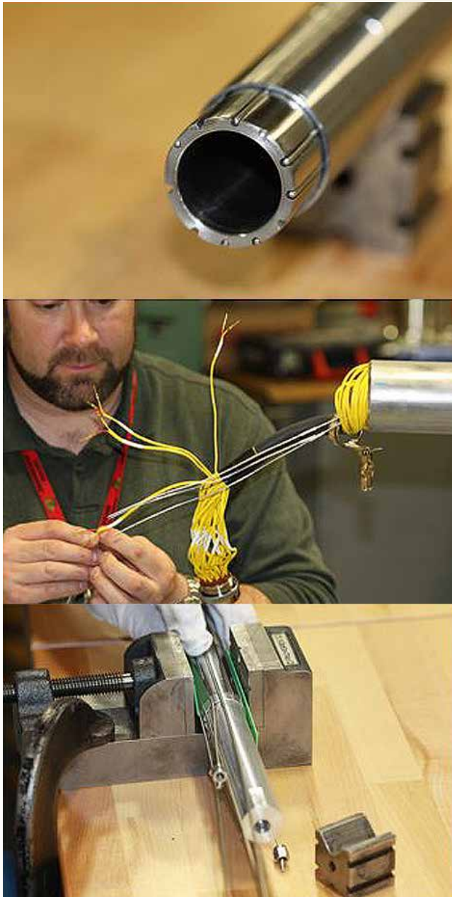
Figure 1. Thermocouple and gas feed assembly.
