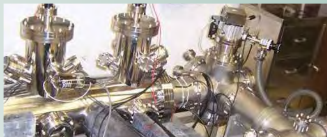
The Positronium Annihilation Lifetime Spectrometer, located in the PULSTAR reactor facility on the NC State North Campus in Raleigh, N.C.
