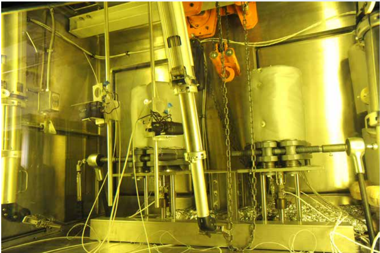
The newly built and installed Irradiation-Assisted Stress Corrosion Cracking (IASCC) test rig at INL's Materials and Fuels Complex is a unique facility that not only has the capacity to conduct examinations of large volumes of materials and full-size specimens, but also can inspect materials that are highly radioactive.
