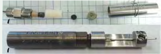
Figure 2. Piezoelectric transducer fabrication. (Top) Transducer components from left to right: stainless steel cap, alumina insulation, nickel plunger, alumina insulation, carbon-carbon backing, Kovar waveguide with zinc oxide sensor on top, stainless steel outer casing. (Bottom) Fully assembled transducer housing with cable and strain-relief sleeve to support the cable connection.
