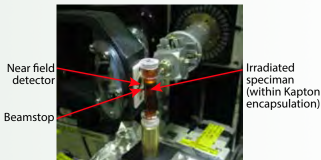
Figure 1. Specimen and detector configuration for HEDM measurements.
