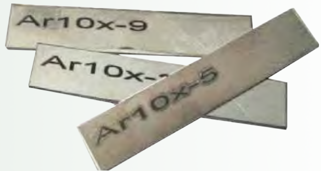
Figure 2. Zirconium specimens used for irradiation and post-irradiation examination.
