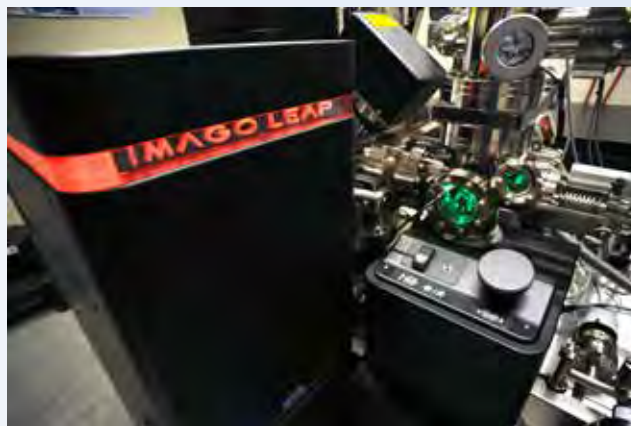
The local electrode atom probe (LEAP) in the Microscopy and Characterization Suite in CAES.
