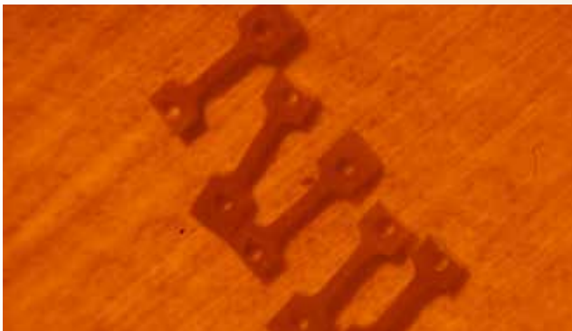
Figure 2. Photograph of tensile specimens sheared during capsule disassembly.
