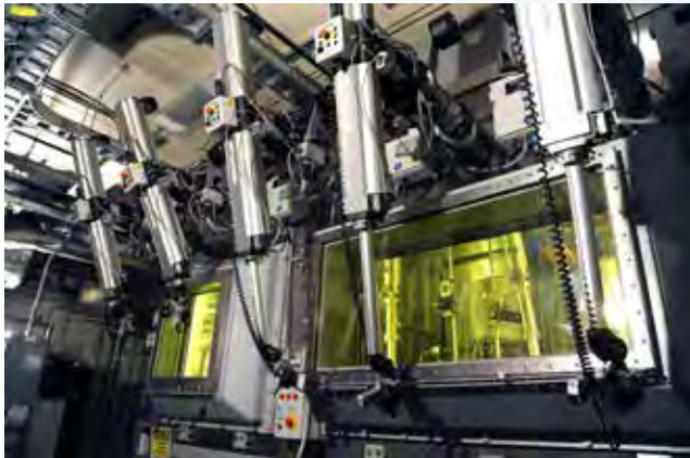
The newly constructed irradiation-assisted stress corrosion crack (IASCC) test rig at INL's Materials and Fuels Complex.
