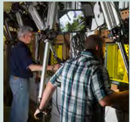
Operators use manipulators to perform work at the Westinghouse Hot Cell Lab.
