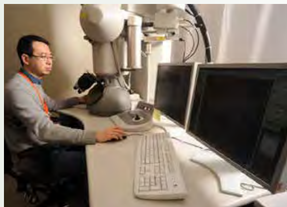
Transmission electron microscope, one of many PIE capabilities in the Microscopy & Characterization Suite (MaCS) at the Center for Advanced Energy Studies in Idaho Falls, Idaho.
