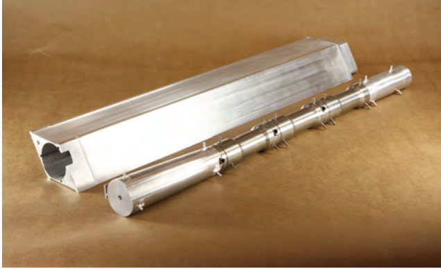
As-fabricated components of the fueled in-core facility before sample installation.
