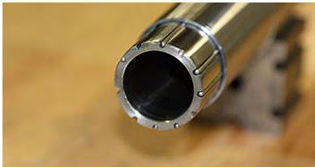
Figure 2. The thermocouple and gas feed assembly.
