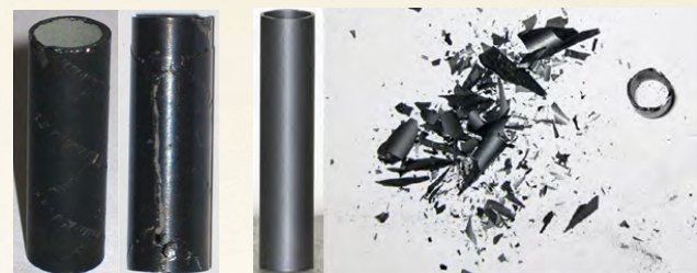
Figure 3. (left two) Round 7 triplex tube before and after expanding plug burst test to failure. (right two) A “monolith-only” tube before and after expanding plug burst test to failure.
