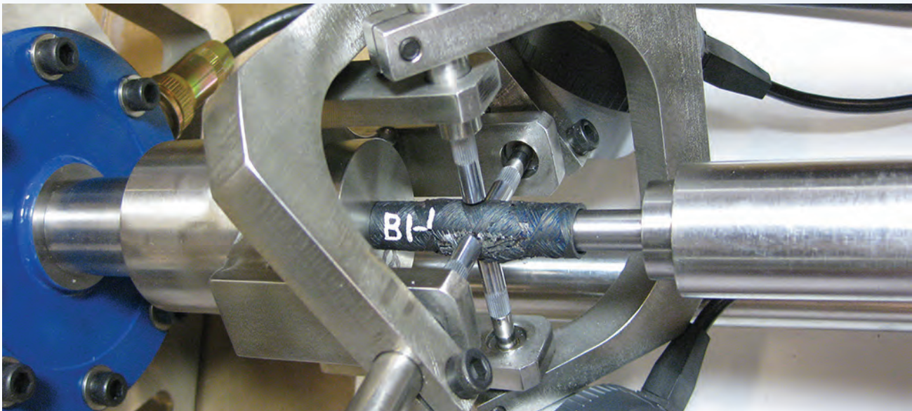
Irradiated SiC/SiC composite clad tube undergoing burst testing.
