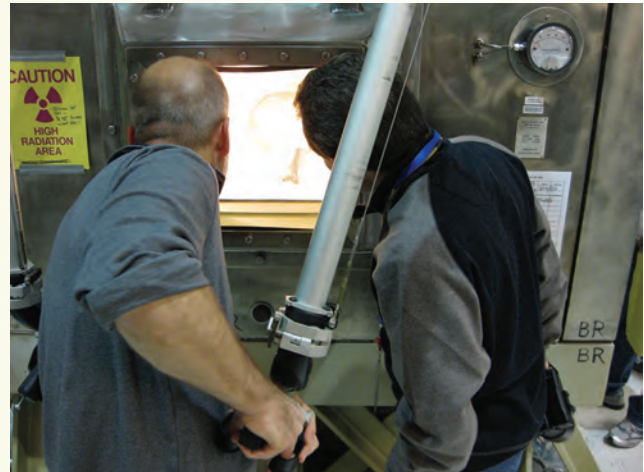
MIT NRL reactor floor hot cell in use for in-core experiment disassembly.
