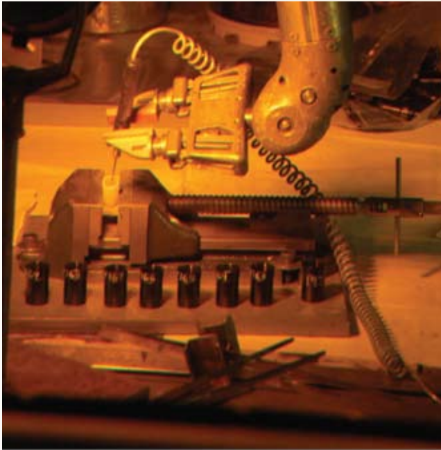
Figure 2. The vacuum removal tool in HFEF removing specimen discs from an irradiation capsule.
