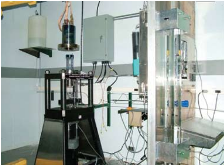
The supercritical water facility in the Irradiated Materials Laboratory, and the schematic of its mobile construction.
