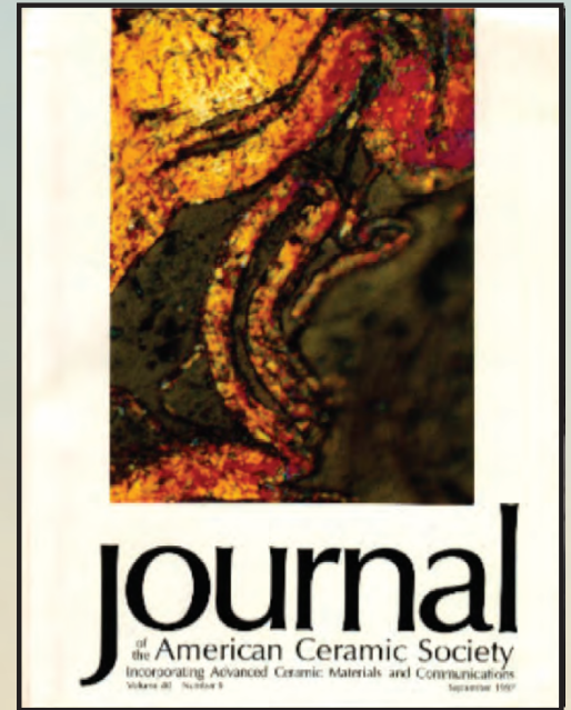
Figure 2. A photo on the cover of the September 1997 issue of Journal of the American Ceramic Society shows the extraordinary extent that individual ultra-large grained Ti_3SiC_2 samples can deform at room temperature.
