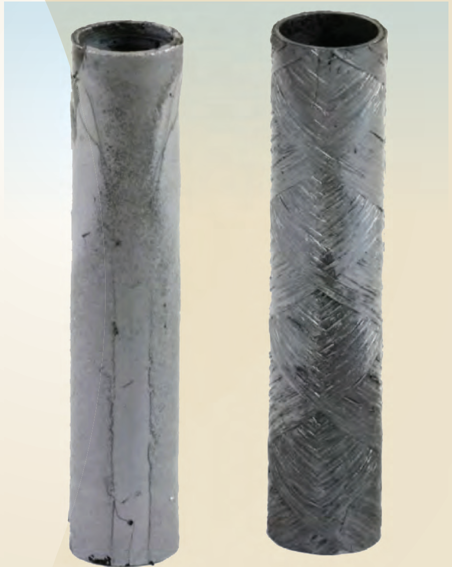
Figure 1. Triplex SiC composite clad tube samples — round 7-generation (near right) and round 6-generation (far right) — after Phase 1 irradiation under pressurized water reactor conditions in an in-core loop at the MIT reactor.
