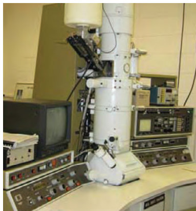
A JEOL 200CX TEM equipped with EDS and scanning system, and an electropolisher and dimpler at the Characterization Laboratory for Irradiated Materials, located on the UW-M campus in Madison, Wis.
