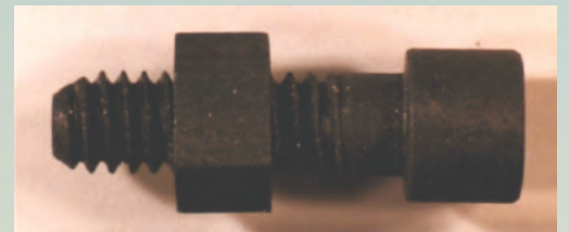
Figure 4. A nut and screw machined out of Ti_3SiC_2 can be cut with a manual hack saw, showing that all the MAX phases are most readily machinable in their final fully dense state.
