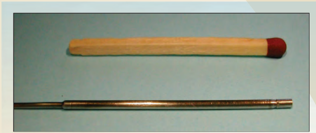
Figure 1. A sub-miniature fission chamber (bottom), a real-time state-of-the-art in-pile flux detection instrument developed by the Commissariat de Energie Atomique, is one of the flux detector technologies that will be assessed at the Advanced Test Reactor. A matchstick is shown as a basis for comparison.
