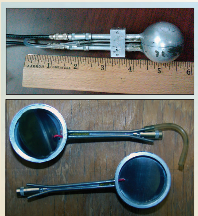
Figure 3. The third type of flux detector that will be assessed is a back-to-back (BTB) fission chamber, shown closed above right and open below.
