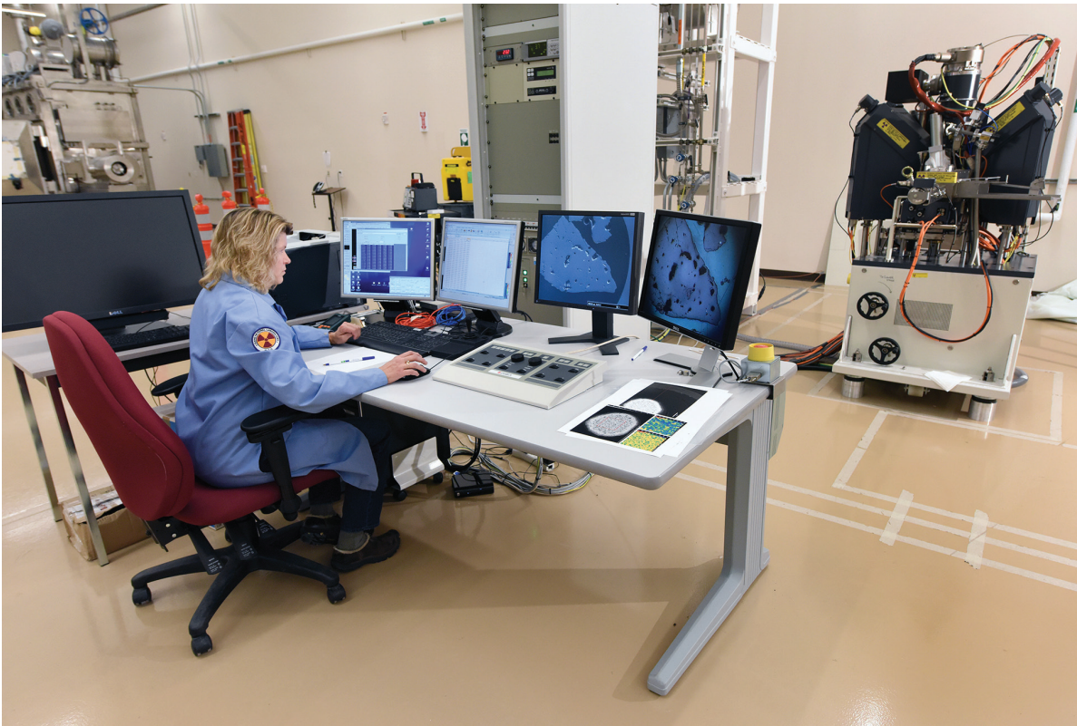
A researcher operating electron probe microanalyzer (EPMA) at IMCL.
