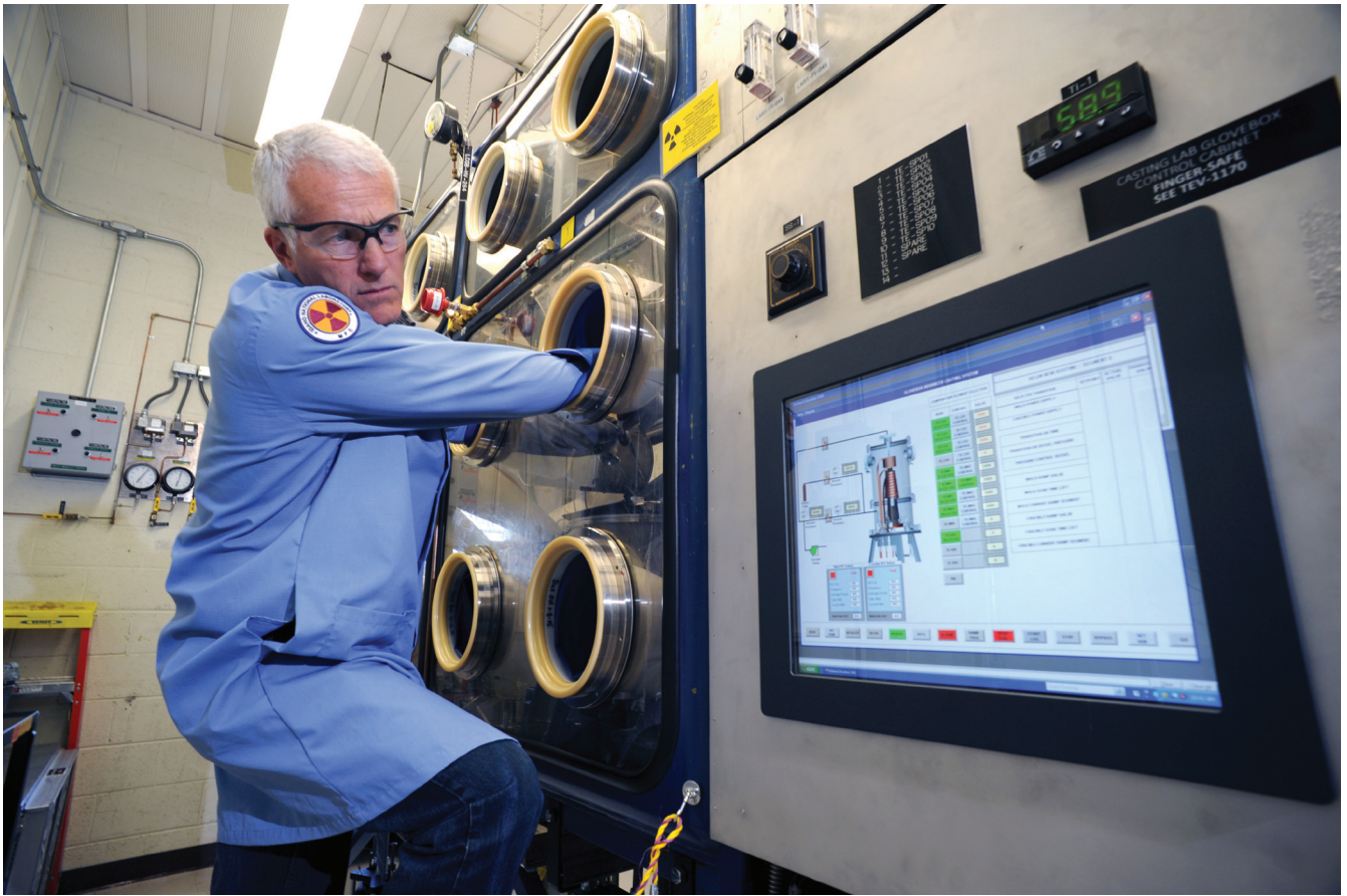
An INL researcher works in the casting lab glove box in MFC's Analytical Laboratory.
