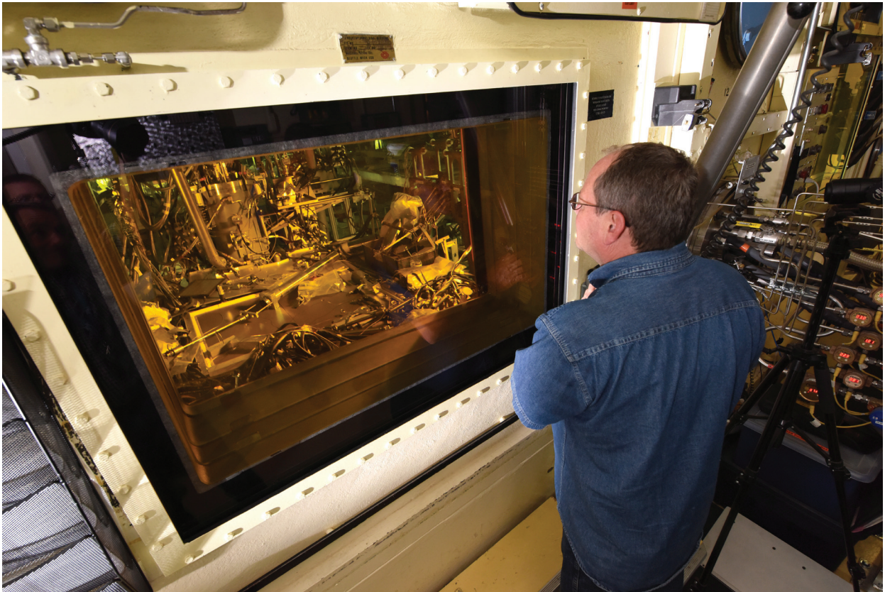
An operator using manipulators at the Hot Fuel Examination Facility.
